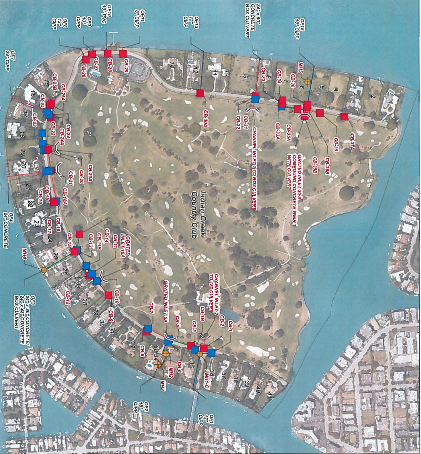
Figure 1: Existing Stormwater Infrastructure November 2018
