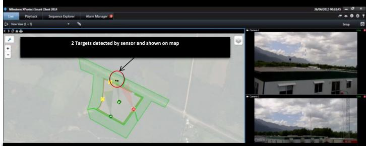
PTZ Cameras Auto-cued to sensor detections If there's more than 1 detected target system decides on optimal PTZ to be sent to view target
